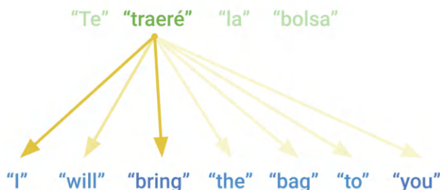
Figure 15.4 Attention assigns a relevance score to each vector in a source for each vector in a target sequence.
