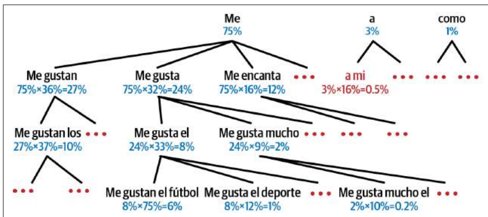
Figure 16-6. Beam search, with a beam width of 3
