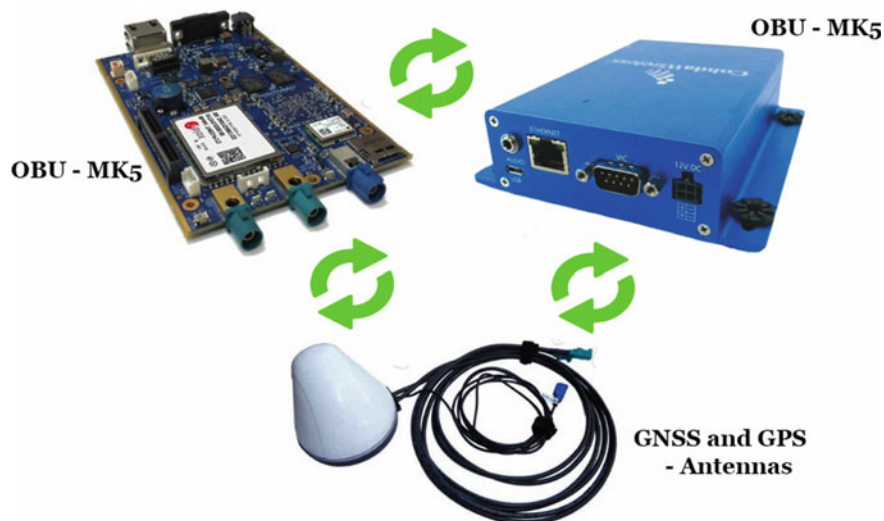
Fig. 11.3 Illustration regarding the hardware structure of some MK5—OBU modules, but also of the GPS-GNSS antennas
