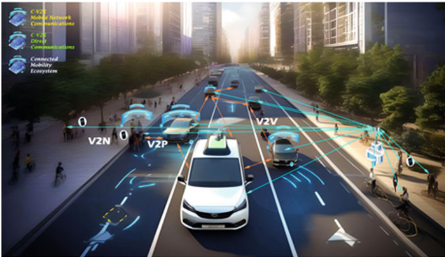
Fig. 11.1 Vehicle-to-everything (V2X) is a connected mobility platform that allows vehicles to interact with their surroundings, such as other vehicles, cyclists, pedestrians, road infrastructure or mobile networks
