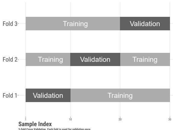
Figure 10.5: Three-fold cross-validation.
