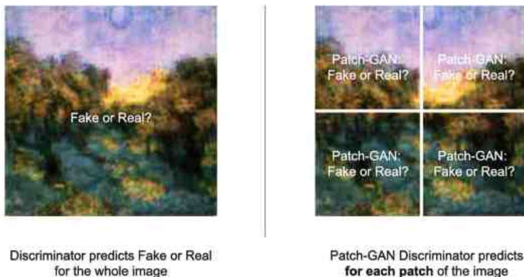
Fig 13.5: Simplified illustration to understand the working of a PatchGAN discriminator
