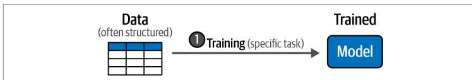
Figure 1-29. Traditional machine learning involves a single step: training a model for a specific target task, like classification or regression.
