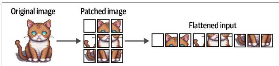
Figure 9-4. The “tokenization” process for image input. It converts an image into patches of subimages.
