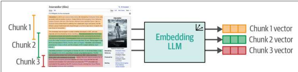
Figure 8-10. Chunking the text into overlapping segments is one strategy to retain more of the context around different segments.
