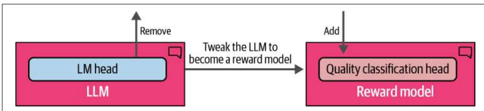
Figure 12-25. The LLM becomes a reward model by replacing its language modeling head with a quality classification head.
