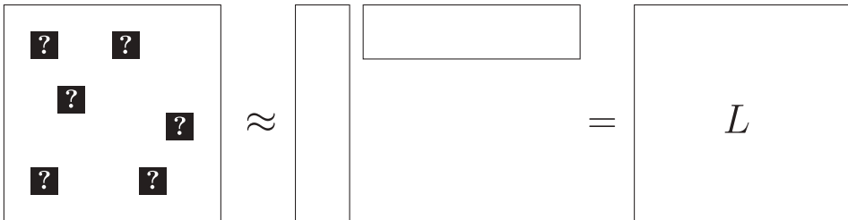
Figure 11.25 Low-rank matrix completion. The diagram shows how to leverage low-rank models to estimate the missing entries in a matrix. The parameters of the model are estimated using the observed data, and then used to form the low-rank estimate L , which provides an estimate of the unobserved entries.
