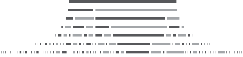
Figure 5.5 An example of a process giving rise to a log-normal distribution. A glass rod breaks into two n times. Each break happens at a random position. Notice that the final lengths vary very considerably.
