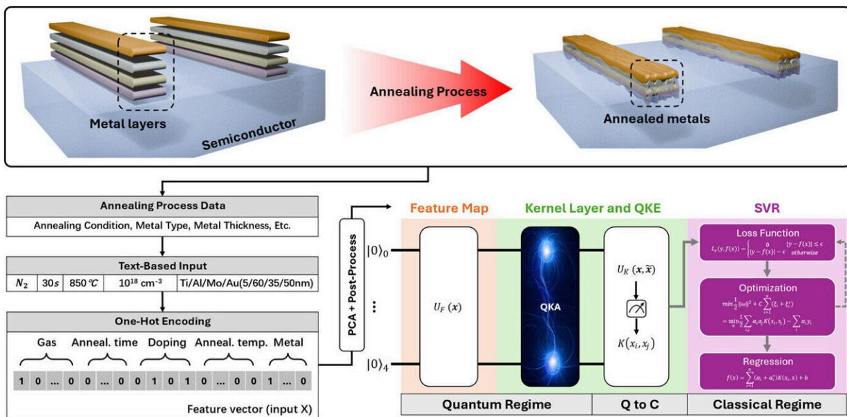
Schematic representation of the quantum machine learning-based modeling process for the Ohmic contact formation in GaN HEMTs. Credit: *Advanced Science* (2025). DOI: 10.1002/advs.202506213
