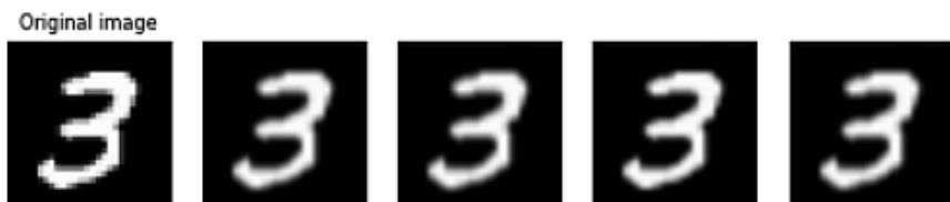
Figure 7.6 – The results of applying the `GaussianBlur` function on the image
