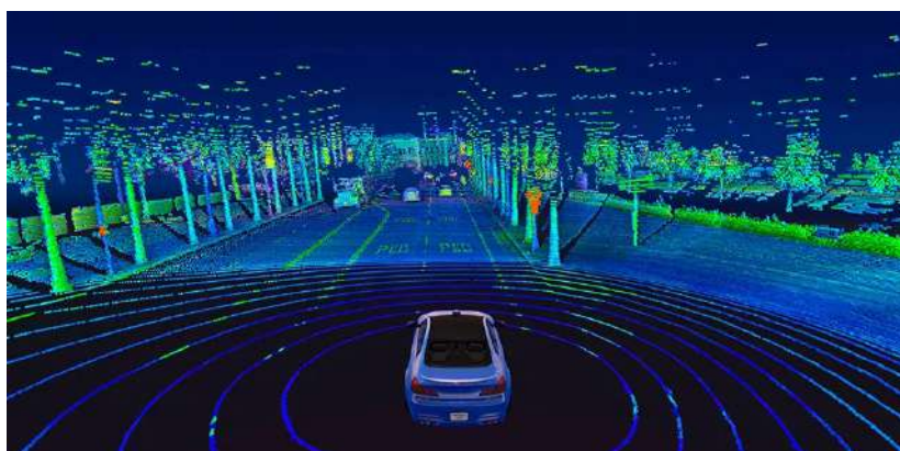
Fig. 2. A lidar point cloud created by Velodyne lidar.
