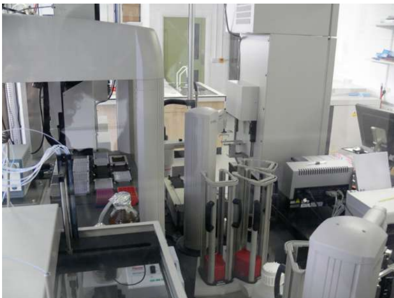
Fig. 1. Adam Robot Scientist. Adam is a computer system that fully automates the scientific process. Within limits, he can come up with new hypotheses, design, and carry out experiments to test them.
