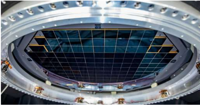
Fig. 1. The focal plane for the Rubin LSST camera. The camera comprises 189 sensors with a total of 3.2 billion pixels. Each image from the camera can be read out in two seconds and, combined with the Rubin telescope, covers approximately 10 square degrees of the sky (credit: Jacqueline Orrell/SLAC National Accelerator Laboratory).
