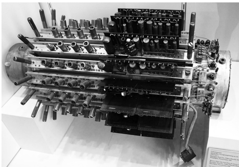
Figure 6.4: Pulses of sound bounced back and forth in the UNIVAC’s “mumble-tub” mercury delay line memory.
