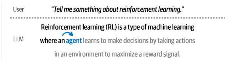
Figure 12-2. During supervised fine-tuning, the LLM aims to predict the next token based on an input that has additional labels. In a sense, the label is the user's input.
