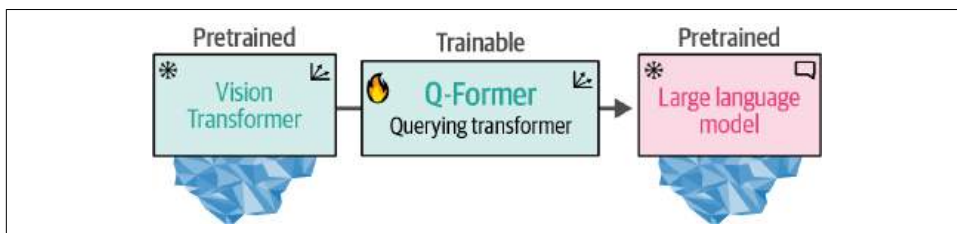
Figure 9-16. The Querying Transformer is the bridge between vision (ViT) and text (LLM) that is the only trainable component of the pipeline.
