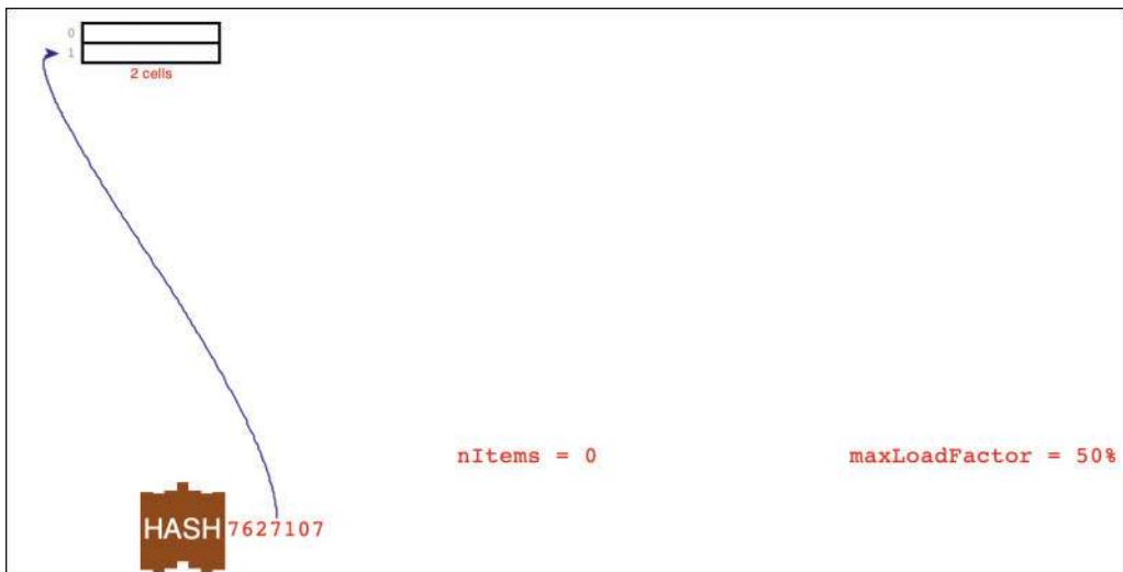
FIGURE 11-7 Probing to insert the key cat in an empty hash table
