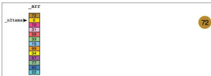
FIGURE 13-9 A random set of items in the array used for the heap
