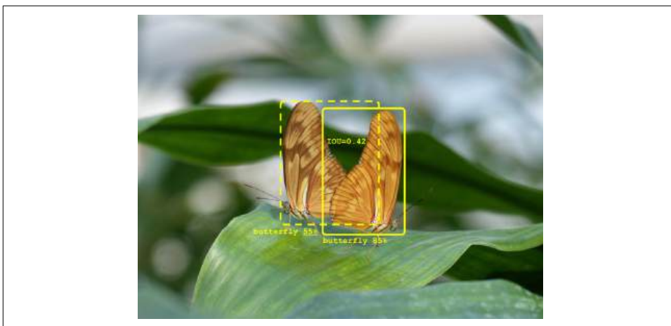
Figure 4-20. Objects close to each other as handled by Soft-NMS. The detection box on the left is not deleted, but its confidence factor is reduced from 78% to 55%. Image from Arthropods dataset .
