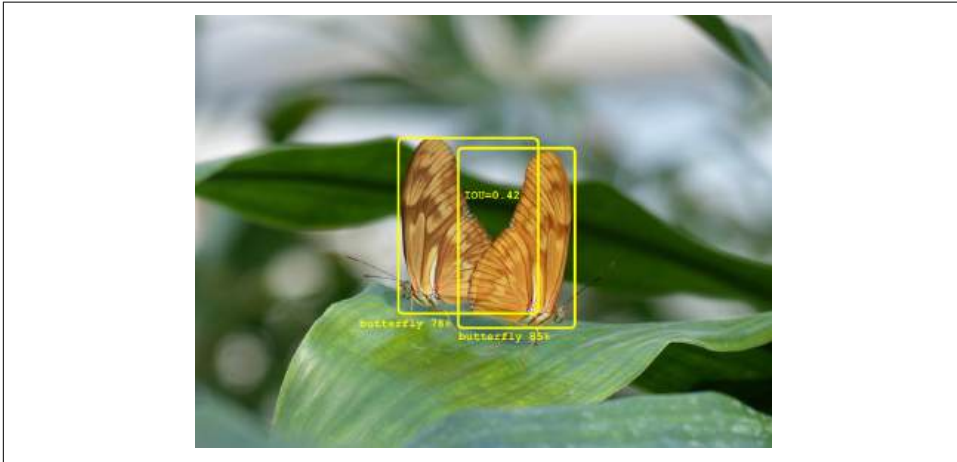
Figure 4-19. Objects close to each other create a problem for the non-max suppression algorithm. If the NMS threshold is 0.4, the box detected on the left will be discarded, which is wrong. Image from Arthropods dataset .
