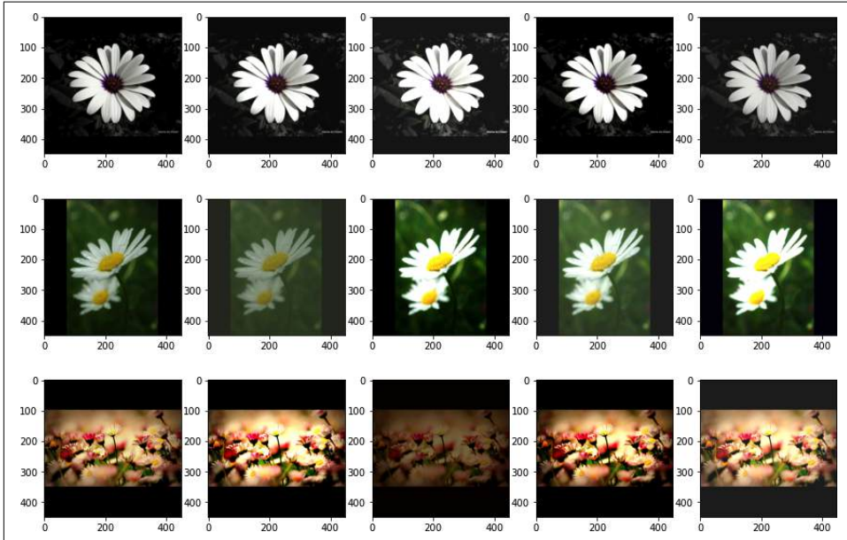
Figure 6-11. Random contrast and brightness adjustment on three of the training images. The original images are shown in the first panel of each row, and four generated images are shown in the other panels. If you're looking at grayscale images, please refer to 06e_colordistortion.ipynb on GitHub to see the effect of the color distortion.
