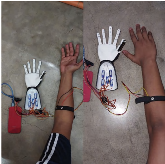
Fig. 1 Electrodes placement for signal acquisition [5]
