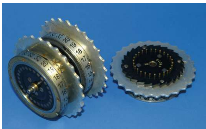
Fig. 8.2 Example of an electromechanical rotor from an Enigma machine (NSA, National Cryptologic Museum)
