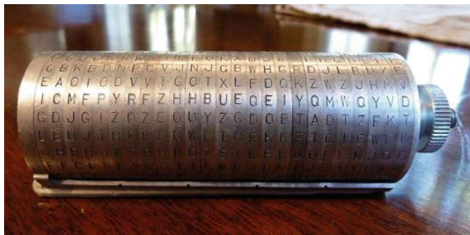
Fig. 8.1 U.S. Army M-94 cipher device (used by permission. Ralph Simpson. CC Attribution-ShareAlike 4.0 International License)
