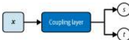
Figure 6-5. A coupling layer outputs two tensors that are the same shape as the input: a scaling factor ( s ) and a translation factor ( t )
