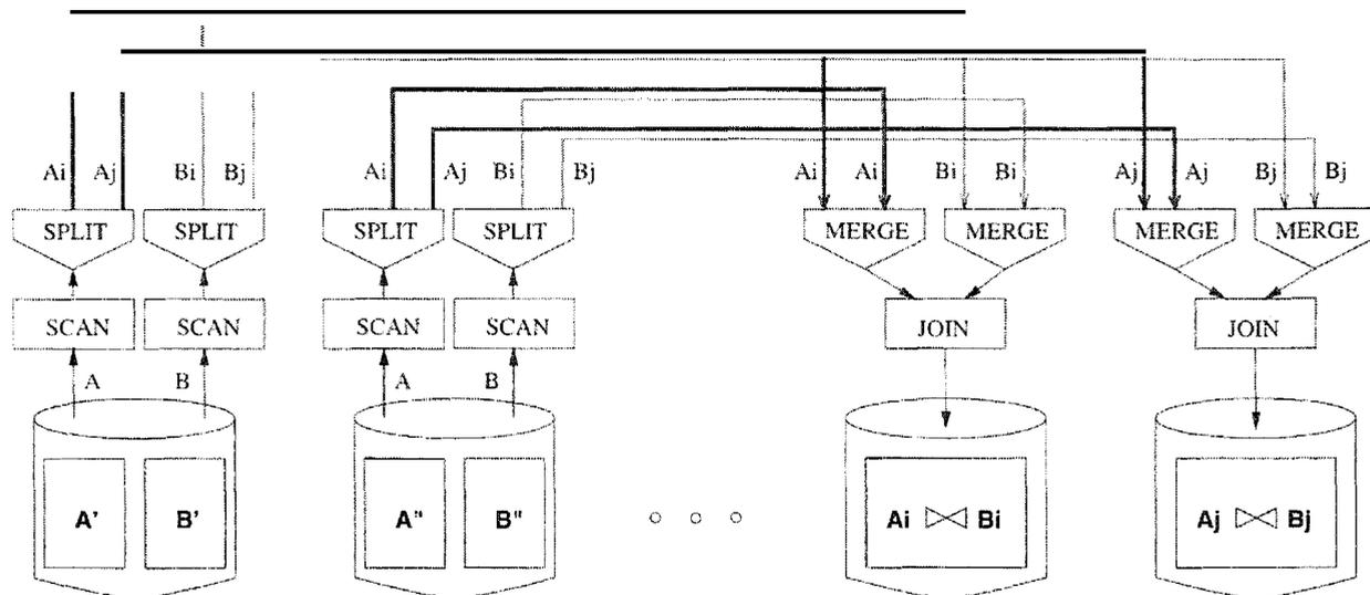
Figure 22.3 Dataflow Network of Operators for Parallel Join
