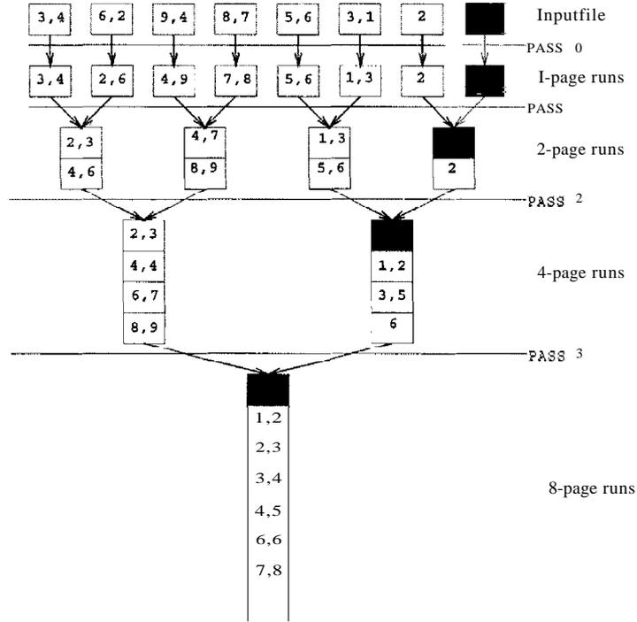
Figure 13.2 Two-Way Merge Sort of a Seven-Page File
