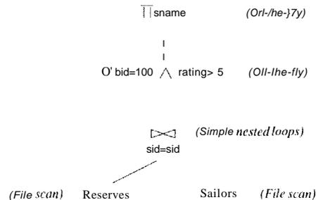
Figure 12.4 Query Evaluation Plan for Sample Query
