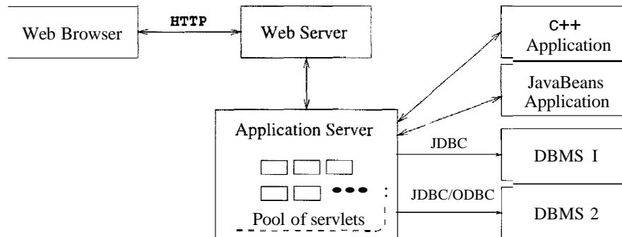
Figure 7.17 Process Structure in the Application Server Architecture
