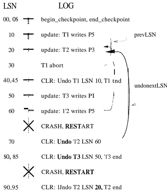
Figure 18.5 Example of Undo with Repeated Crashes
