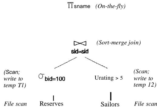
Figure 12.6 A Second Query Evaluation Plan
