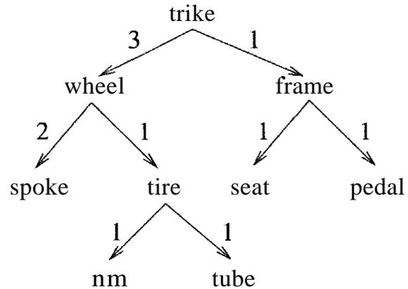
Figure 24.2 Assembly Instance Seen as a Tree
