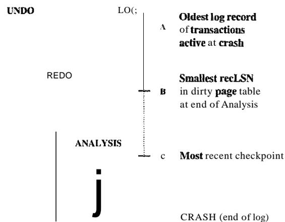
Figure 18.4 Three Phases of Restart in ARIES
