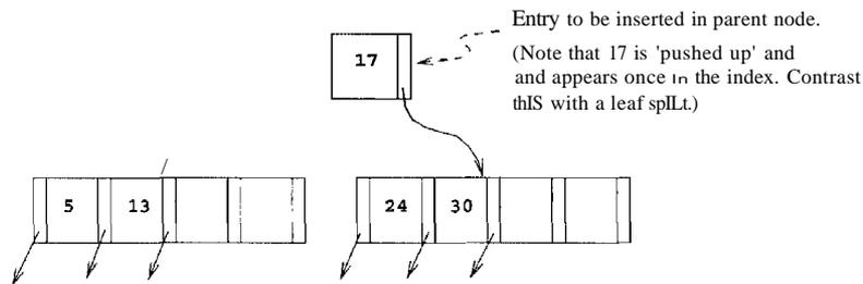
Figure 10.12 Split Index Pages during Insert of Entry 8\*
