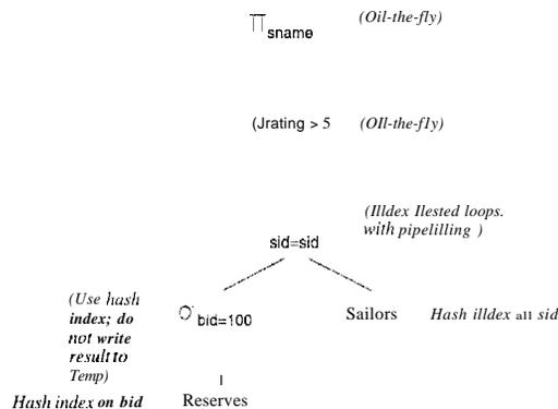
Figure 12.7 A Query Evaluation Plan Using Indexes
