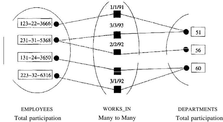
Figure 2.3 An Instance of the Works\_In Relationship Set
