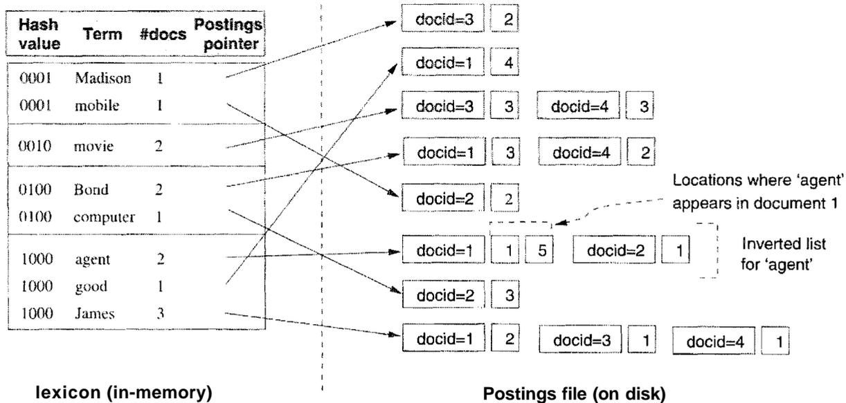
Figure 27.5 Inverted Index for Example Collection
