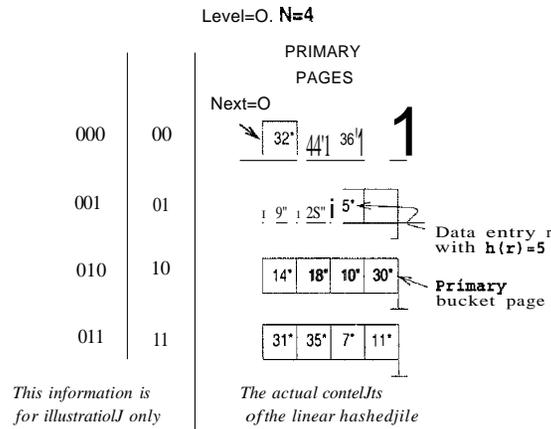
Figure 11.8 Example of a Linear Hashed File
