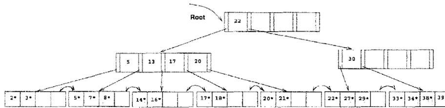
Figure 10.19 A B+ Tree during a Deletion
