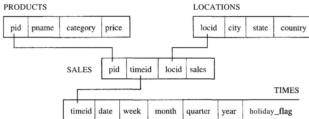
Figure 25.4 An Example of a Star Schema
