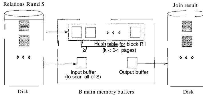
Figure 14.6 Buffer Usage in Block Nested Loops Join
