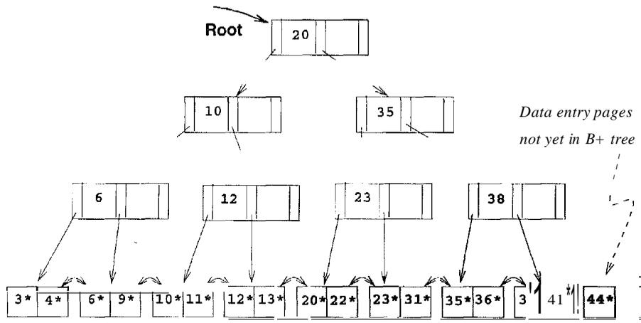
Figure 10.26 After Adding Entry for Leaf Page Containing 38\*
