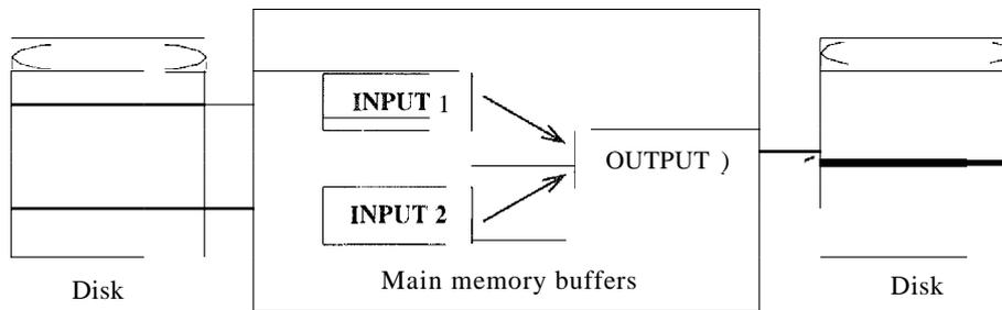
Figure 13.3 Two-Way Merge Sort with Three Buffer Pages
