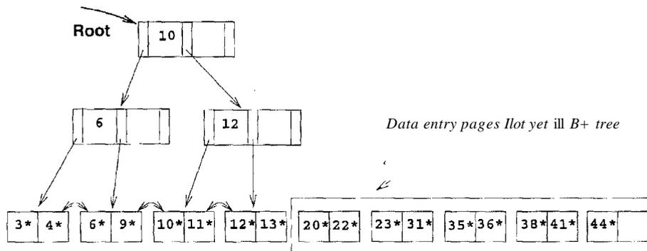
Figure 10.24 Page Split during B+ Tree Bulk-Loading
