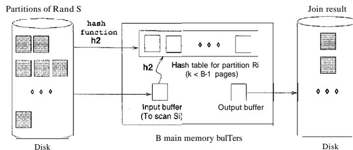
Figure 14.11 Probing Phase of Hash Join
