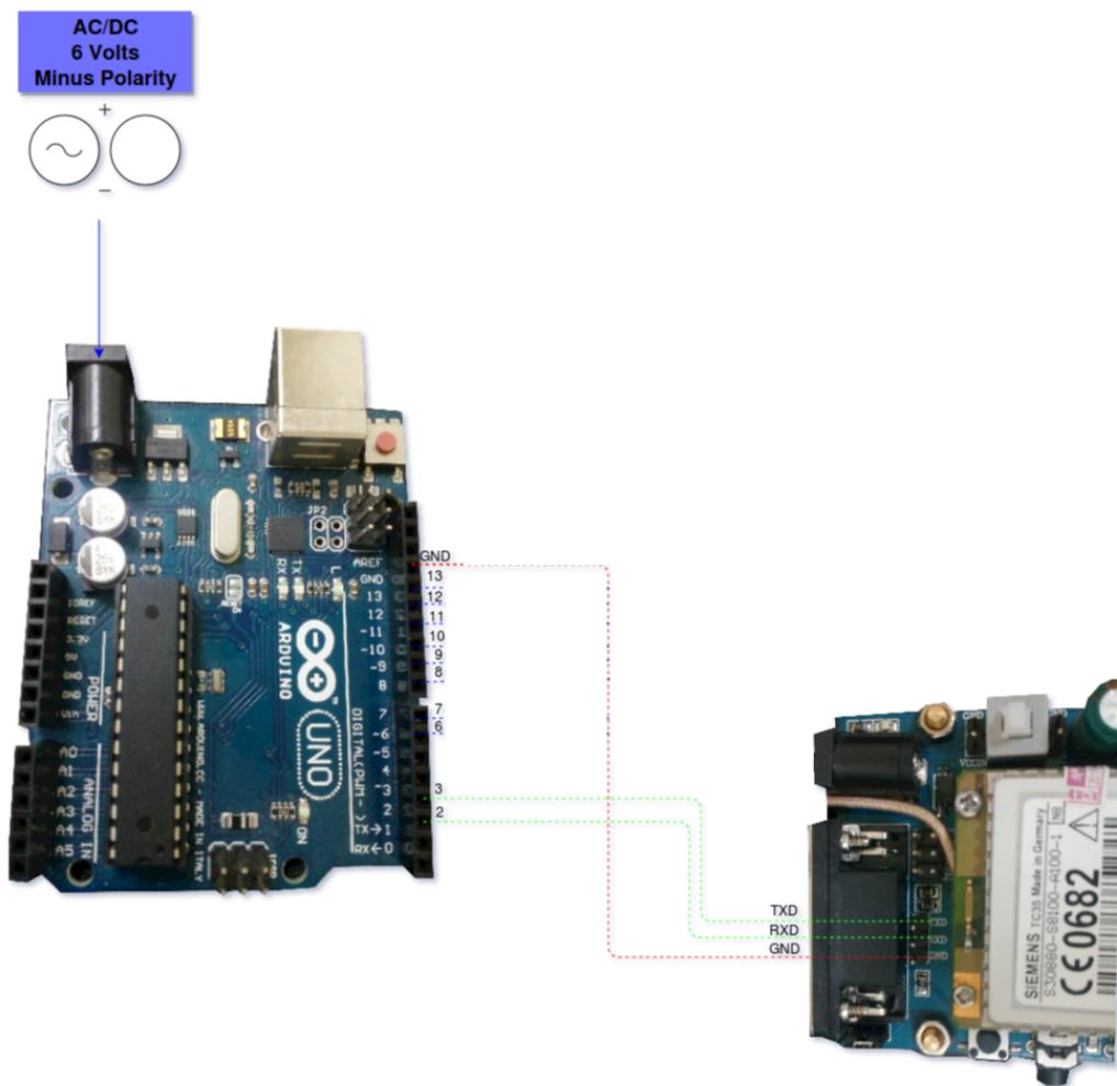
The previous diagram show how the connection between the Siemens TC35 and using TX, RX and GND connection.
