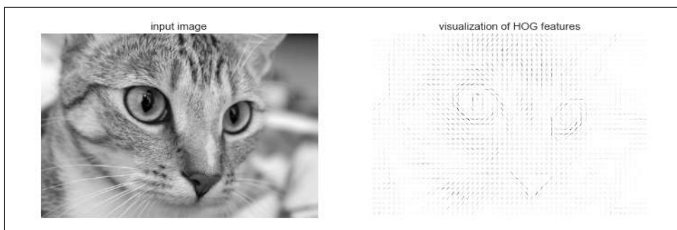
Figure 5-149. Visualization of HOG features computed from an image
