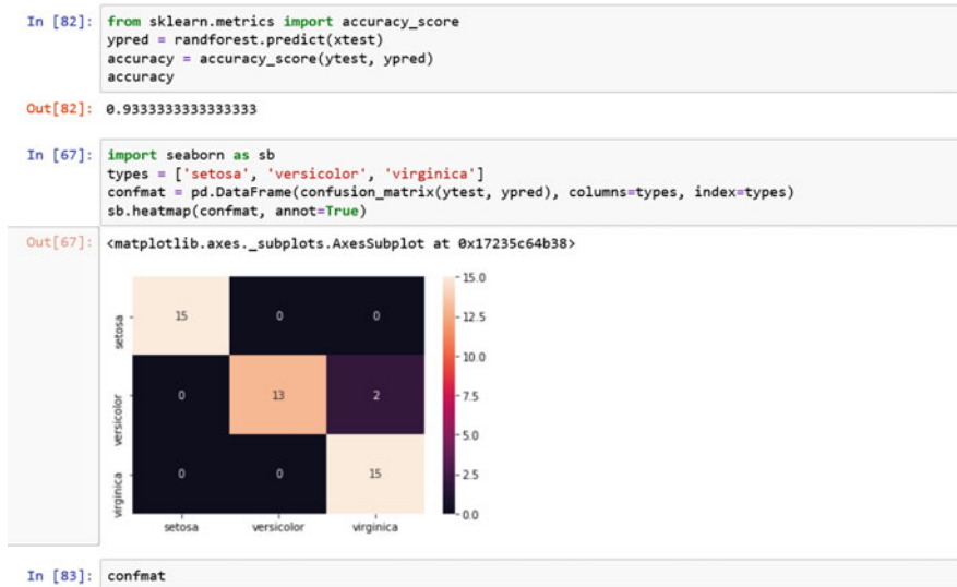
Fig. 23.5 Performance of the classification using metrics of accuracy and confusion matrix
