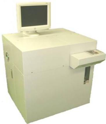
Fig. 4. Photograph of ion trap mass spectrometer using atmospheric pressure ionization mass spectrometer (DS-1000)
